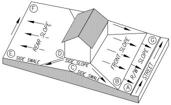
A-B R/W SLOPE 0.03' / FT SLOPE MIN.
